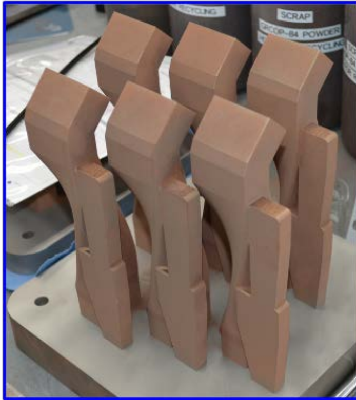
3D printed waveguide structures for the Lower Hybrid system.
