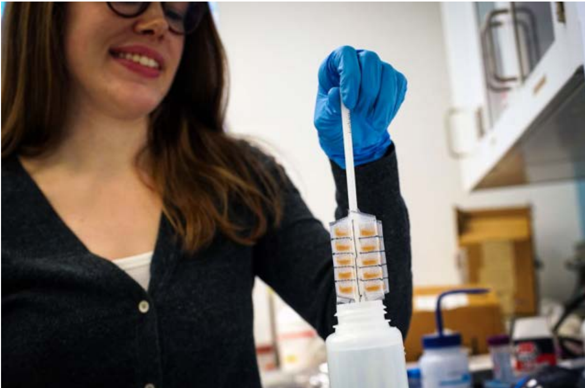
MIT graduate student Emily Hanhauser demonstrates a new device that may simplify the logistics of water monitoring for trace metal contaminants, particularly in resource-constrained regions. (Photo courtesy of Melanie Gonick/MIT)
