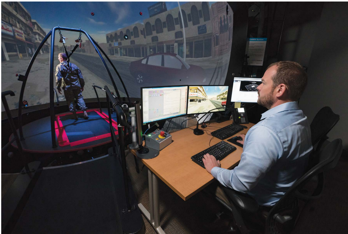
The Sensorimotor Technology Realization in Immersive Virtual Environments Center enables the assessment of cognitive and physiological performance as a person interacts with a virtual environment. The researcher above is monitoring the person's performance.
