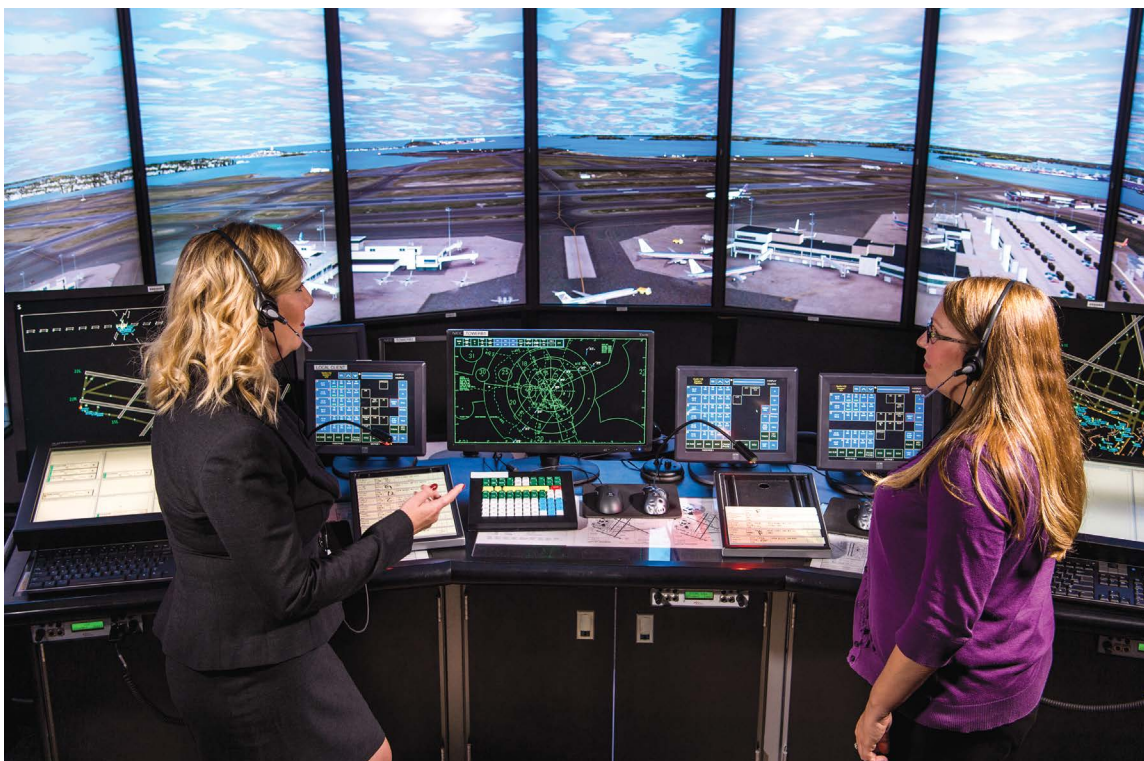
The control tower simulation facility serves as a test bed for evaluating new procedures and technologies that have been developed to improve airport ground operations. Researchers use realistic flight data in their proof-of-concept demonstrations.
