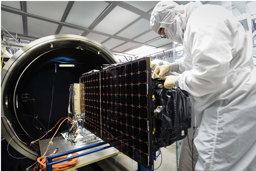
The Operationally Responsive Space-5 SensorSat was delivered to the US Air Force after completion of testing to verify the hardware-to-software interfaces, vibration testing to replicate the launch environment, and performance testing in a thermal-vacuum chamber to simulate the space environment.
