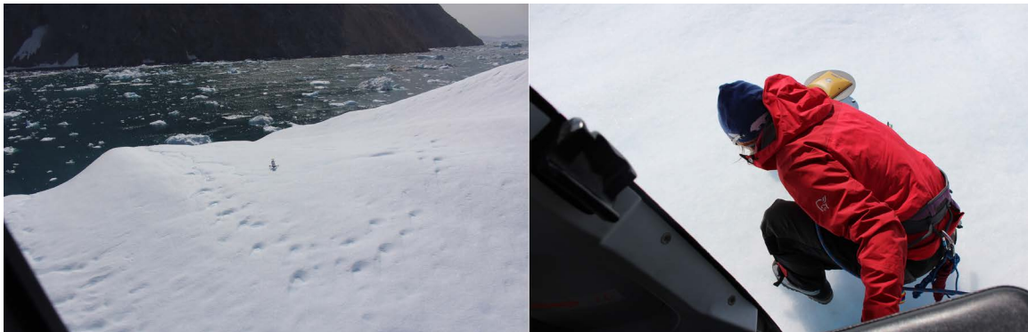
MIT GPS receivers are placed on an iceberg in Sermilik Fjord, East Greenland, to study iceberg melt, meltwater input, and mesoscale ocean circulation.
