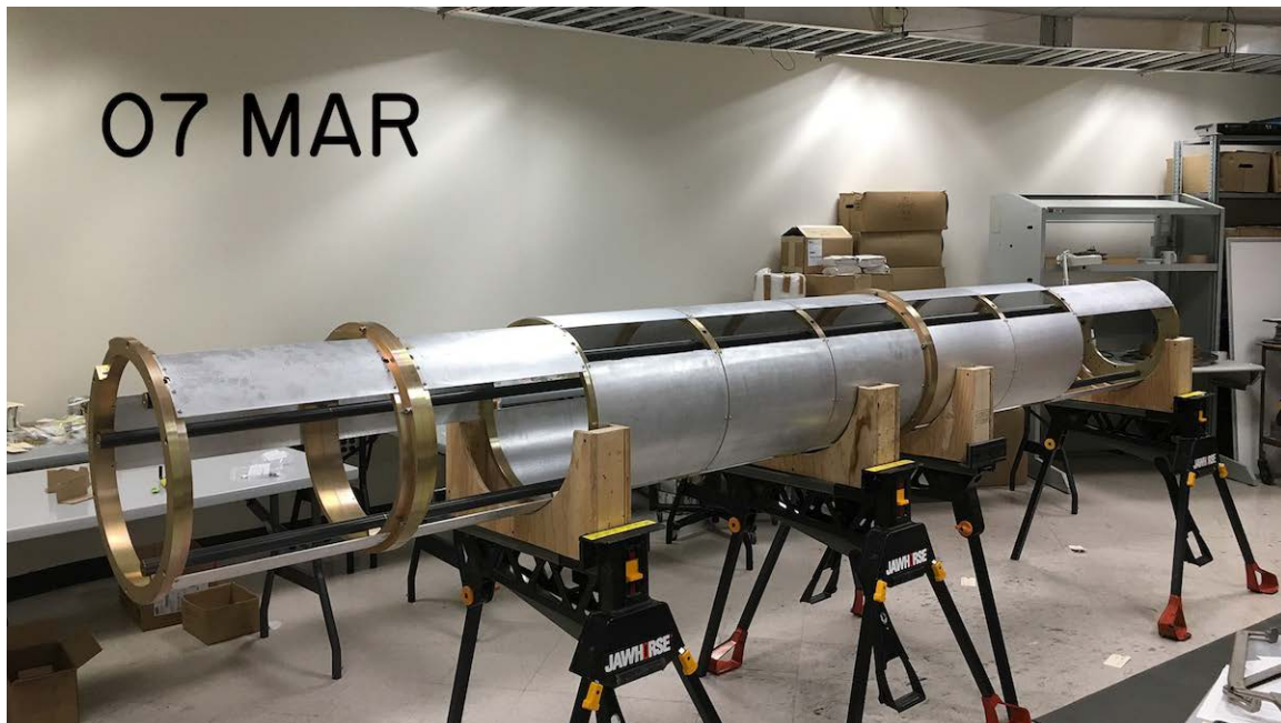
Progress on building the front end of the signal chain for the VGOS telescope at McDonald Observatory in Texas. Shown is the front-end positioner in the Westford technical laboratory in March 2018.
