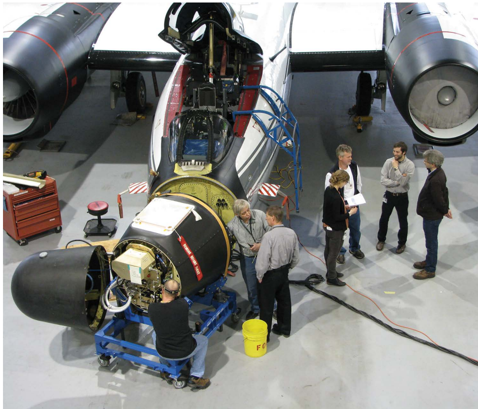
High-precision pointing of an airborne optical terminal requires highly integrated optomechanical designs. These requirements entail close collaboration among mechanical designers, thermal and structural engineers, and optical experts. Here, an optical terminal is being integrated into a high-altitude WB-57 aircraft for pointing and navigation testing.
