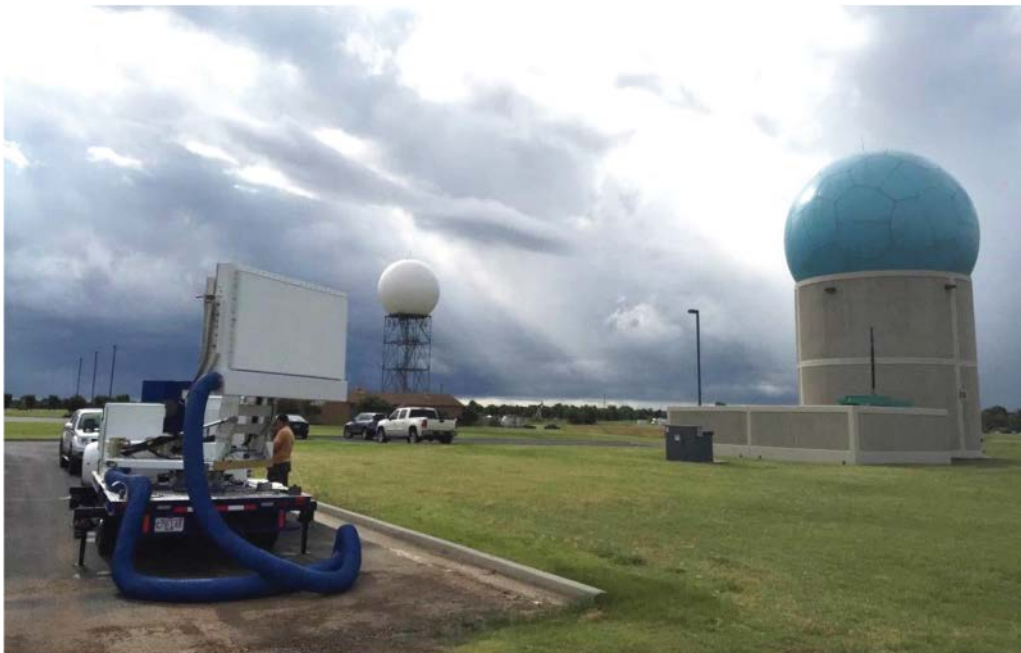
The laboratory developed the portable 10-panel MPAR prototype (left), which was deployed to the National Severe Storms Laboratory in Norman, OK. Work continues on a full-scale 76-panel Advanced Technology Demonstrator array, which will be installed in the blue radome (right). The Advanced Technology Demonstrator will be used in conjunction with a nearby next-generation radar site to collect weather data.
