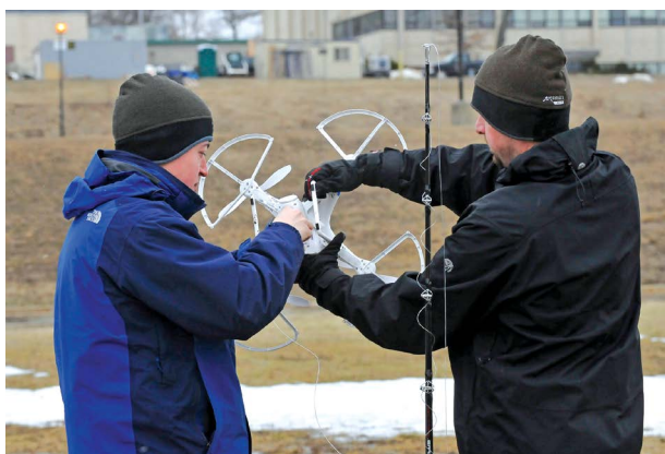
Figure 10. In an effort to develop technology for detecting and tracking UAVs, researchers measure the acoustic signature of a commercial UAV in an urban environment.
