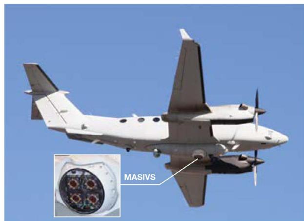
Figure 7. The Lincoln Laboratory MASIVS sensor is fully integrated onto the US Army Constant Hawk aircraft.
