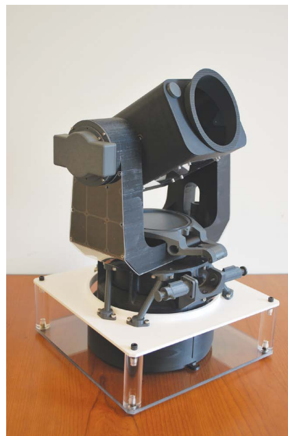
Figure 5. Engineering model of a laser communications terminal.
