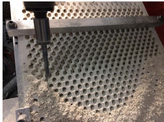
Figure 6: A layer of ceramic being drilled to create a double gyroid photonic crystal for MIT's Institute for Soldier Nanotechnologies, used to observe Weyl points. Each of the 588 holes in the layer is drilled at two different angles; a third angle results from machining 27 grooves in the surface of the layer. The finished photonic crystal consists of 18 such layers.
