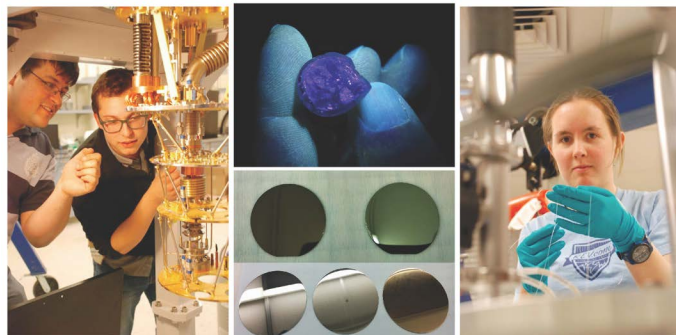
Figure 3: A collage of photos from scintillating bolometer research and development work: (left) a graduate and an undergraduate student install sensors in the dilution refrigerator; (top) crystal test growth of ZnMoO_4 at RMD Inc.; (bottom) anti-reflective coatings for silicon light sensors; (right) an undergraduate student installs calibration fiber in the dilution refrigerator.
