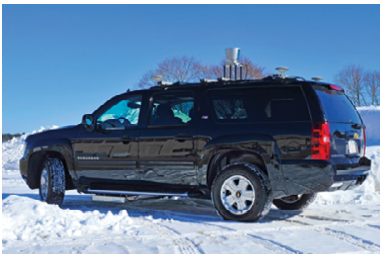
Figure 12. The Laboratory's new ground vehicle test bed is supporting current and future unmanned autonomous systems work in localization, perception, and mapping. A novel Lincoln Laboratory-designed localizing ground-penetrating radar positioned under the vehicle enables three-centimeter-level real-time localization to a prior map at travel speeds of up to 60 mph. A lidar mapping sensor, camera, and dual differential global positioning systems were also integrated into the mobile test bed to provide accurate mapping and localization capabilities.
