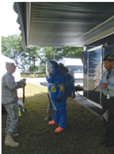
Figure 10. Protective equipment for avoiding heat casualties from chemical, biological, radiological, nuclear, and explosive threats is field tested with the Massachusetts National Guard 1st Civil Support Team at Hanscom Air Force Base.
