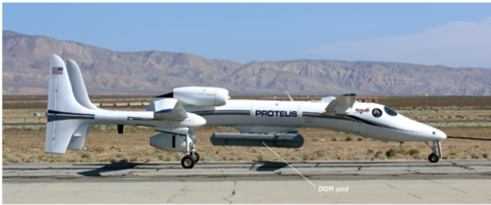
Figure 7. Lincoln Laboratory helped to define an open-systems architecture and supported the development of advanced algorithms for the US Air Force's Dismount Detection Radar (DDR) prototype. The DDR pod was integrated onto a Scaled Composites' Proteus aircraft and underwent development testing at the Mojave Air and Space Port and Edwards Air Force Base in southern California.
