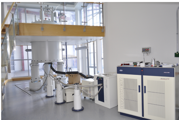
Figure 6. The 900 MHz NMR spectrometer system at PSFC's Francis Bitter Magnet Laboratory.
