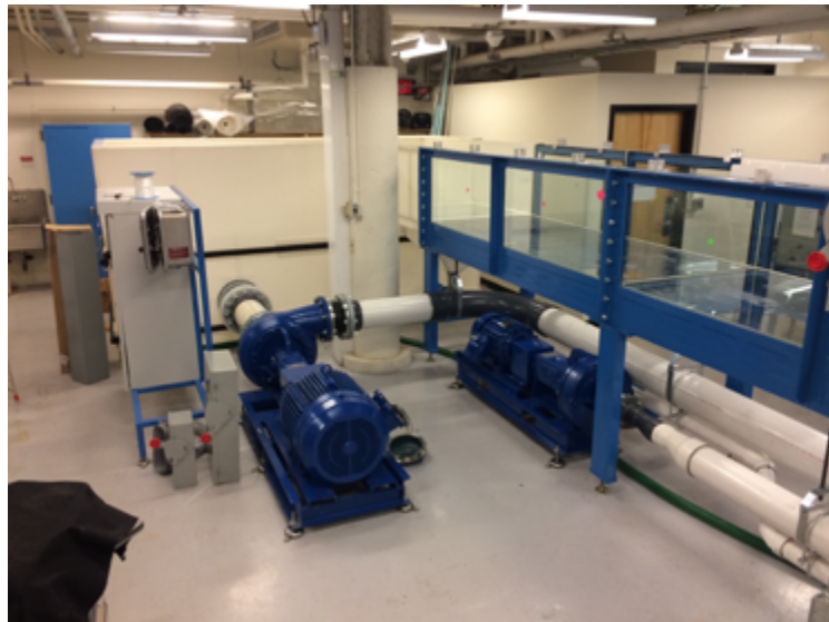
Figure 5: A sediment flume tank made in the Central Machine Shop for Prof. Nepf's lab in MIT's Department of Civil and Environmental Engineering, to study sediment transport in vegetated channels.
