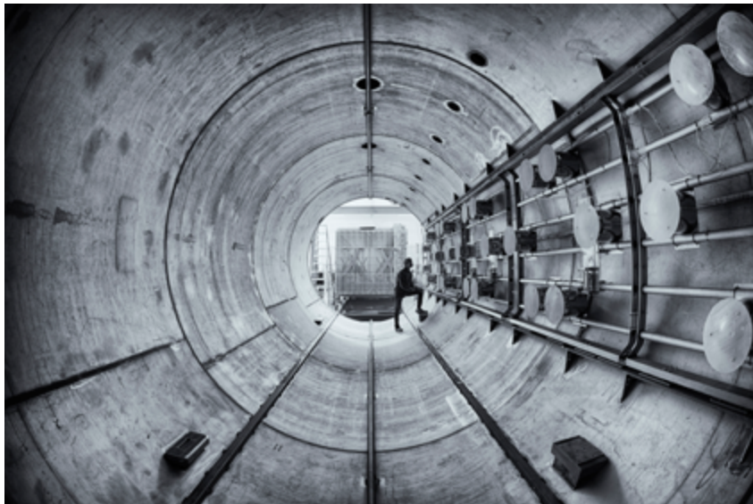
Figure 1: The cryostat for the MicroBooNE liquid argon time projection chamber (LArTPC) during installation of the last wavelength-shifting plate in front of the light collection phototubes (along the right side of the cylinder), before insertion of the LArTPC (background).
