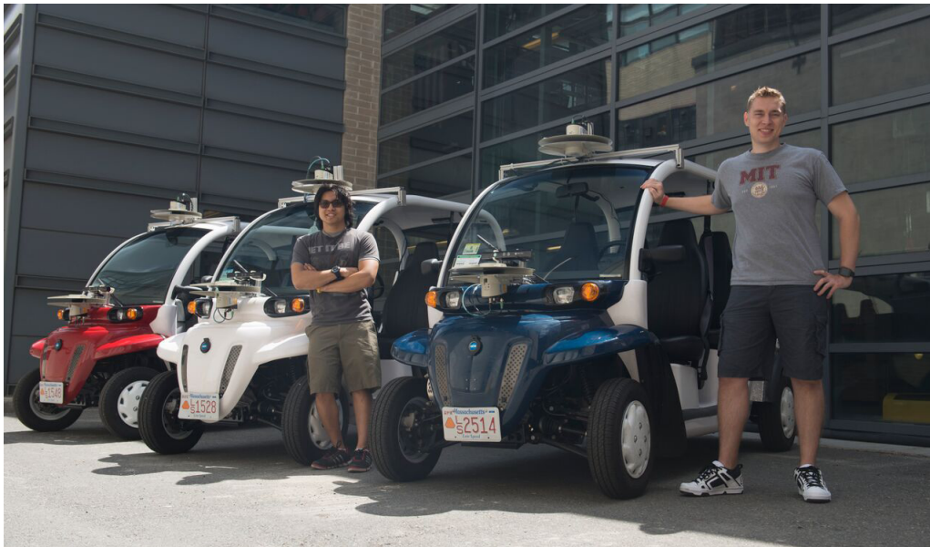
Aerospace Controls Laboratory undergraduate student Wally Wibowo (left) and graduate student Justin Miller in front of AeroAstro's Newman Hangar with vehicles that the laboratory has outfitted with sensors of the type used in self-driving cars. This project, part of the Ford-MIT Alliance, aims to predict pedestrian behaviors on short time scales while providing data to support a mobility-on-demand system for the MIT campus. (Photo: William Litant/MIT)
