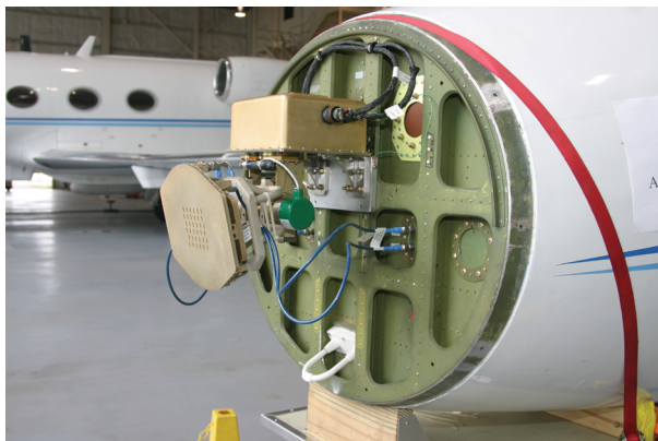
Figure 4. The gimbaled slotted planar array in the Gimbaled Airborne Test Radar test bed collects coherent range-Doppler measurements to demonstrate and evaluate the performance of advanced radar tracking and discrimination performance algorithms. The team that developed this radar was honored with a Lincoln Laboratory Team Award in 2014.
