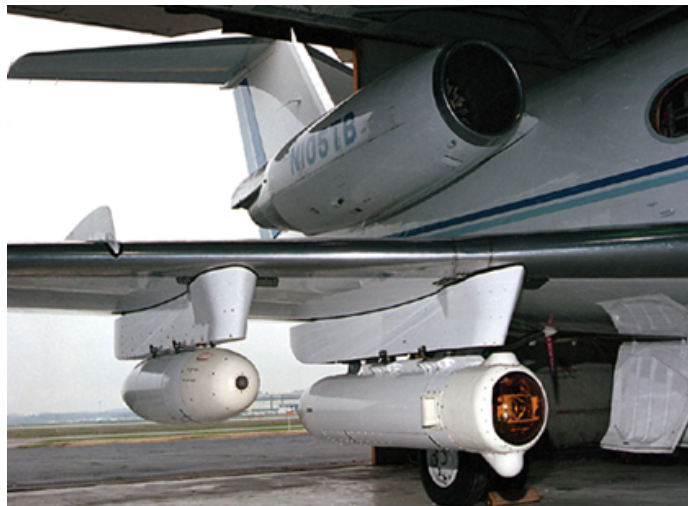
Figure 9. The dual-band, pod-mounted sensor developed for the Airborne Seeker Test Bed is used for airborne infrared imaging and data collection.
