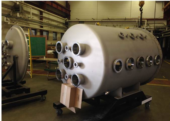
The vacuum chamber for the 1 \text{ m}^3 Dark Matter Time Projection Chamber detector, with the chamber end cap to the left.
