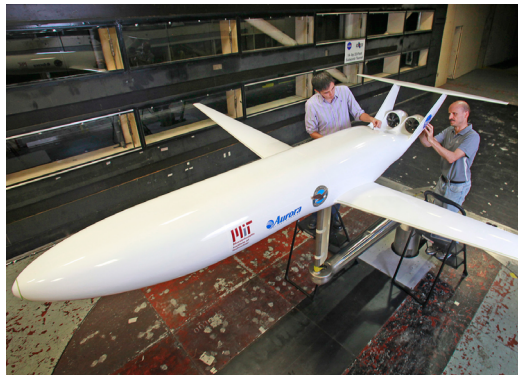
Professor Mark Drela and research scientist Uranga Alejandra prepare a model of the MIT-designed D-8 aircraft for testing in NASA's Langley, Virginia wind tunnel. A 737-size commercial aircraft design, the D-8 has the potential of achieving a 70 percent reduction in fuel use compared to current aircraft
