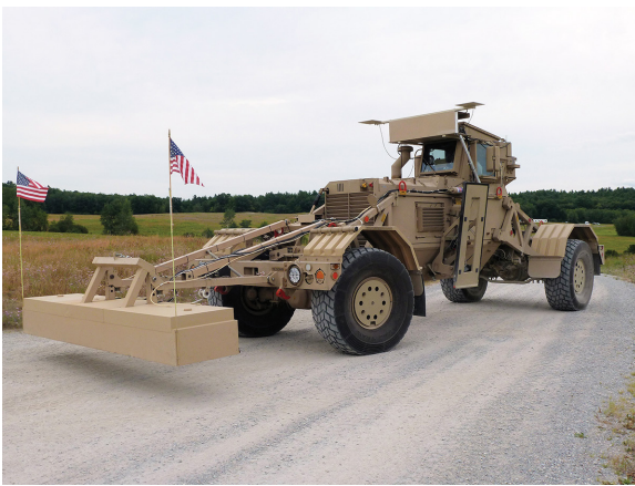
Figure 10. Lincoln Laboratory is developing a novel ground-penetrating radar capability to be used by combat engineers. An initial prototype has been integrated onto an Army Husky vehicle.
