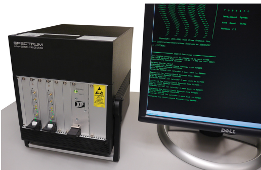
Figure 11. The next-generation airborne collision avoidance system, ACAS X, initial hardware prototype has undergone bench testing.
