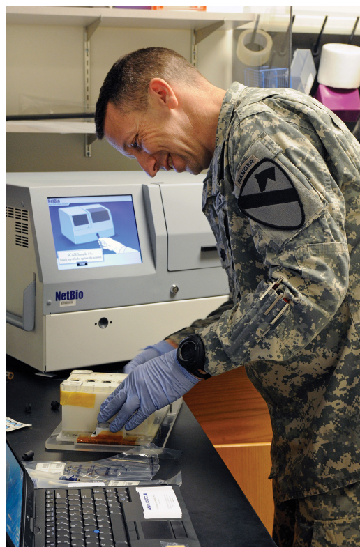
Figure 9. US Army Lieutenant Colonel Scott Jackson, a participant in the Laboratory's Military Fellows Program, loads DNA samples for processing in the accelerated nuclear DNA equipment prototype instrument. The microfluidic-based system is designed to be operated by technicians in expeditionary laboratory facilities to enable rapid, accurate human identification.
