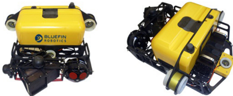
Figure 1: Small, hovering AUVs designed for inspecting ship hulls for explosives or contraband.
