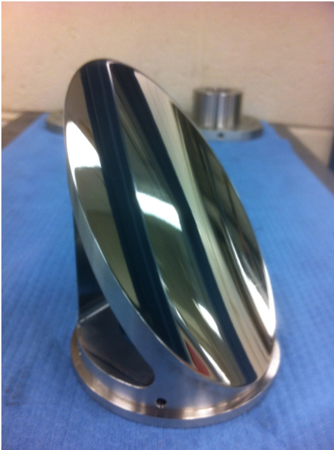
Figure 4. A stainless steel parabolic mirror for MIT's Alcator C-mod tokamak, made in the Central Machine Shop.
