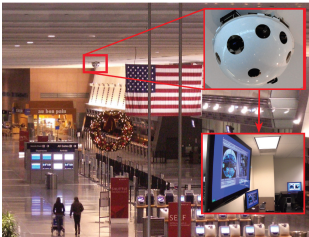
Figure 8. The Imaging System for Immersive Surveillance (top right inset) was tested at Boston's Logan International Airport. The video is displayed in real time (lower right inset).
