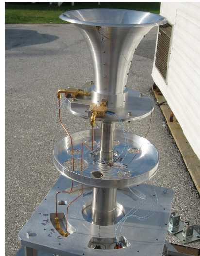
Figure 4. The “quadridge” feed horn being developed and tested for the VLBI 2010 geodesy system at Haystack. This horn is being adapted for geodesy use through a collaboration with Caltech.
