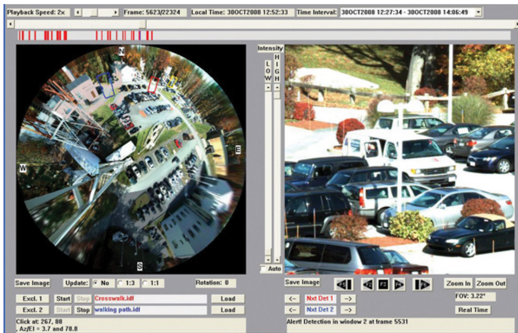
Figure 8. The ISIS display provides 360-degree situational awareness as well as zoomed-in views of a location under surveillance.
