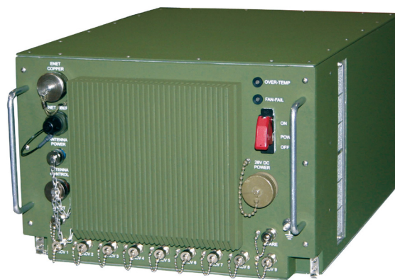
Figure 10. Lincoln Laboratory developed and successfully tested this multichannel signals intelligence receiver, which has enabled the Laboratory to rapidly innovate, develop, and test novel sensor capabilities for a variety of critical national problems. Key features include low noise figure, wide bandwidth, and direction-finding capability.
