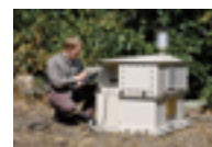
Figure 8. The Rapid Agent Aerosol Detection Program is developing technology for high-performance, lightweight, integrated chemical and biological aerosol detection. Field trials showed reduced false-positive rates and higher agent sensitivity over prior-generation detectors.
