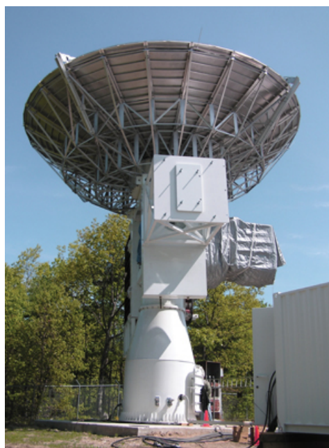
Figure 4. An X-band radar (XTR-1) will be integrated on a ship to support missile-defense testing in the broad ocean area.
