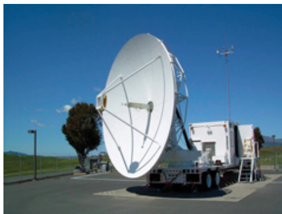
Figure 5. The Large-Aperture Ka-Band Test Terminal was used to perform early characterization of the first Wideband Global System satellite communications payload.
