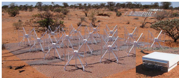
Figure 1. Three antenna tiles of the MWA are visible in this photo from the MWA site in Western Australia. Each tile consists of 16 individual dual-polarization dipoles. In the lower right is a photo of the beamformer that allows the tile beam to be pointed in any direction in the sky.
