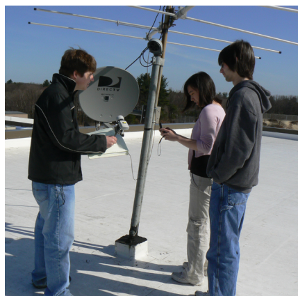
Figure 7. High school students from Chelmsford High School evaluating their ozone spectrometer system, which is based on the VSRT system developed at Haystack Observatory.
