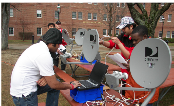
Figure 6. Students at the Middlesex Community College in Bedford, MA, use the VSRT interferometer to measure the diameter of the Sun.
