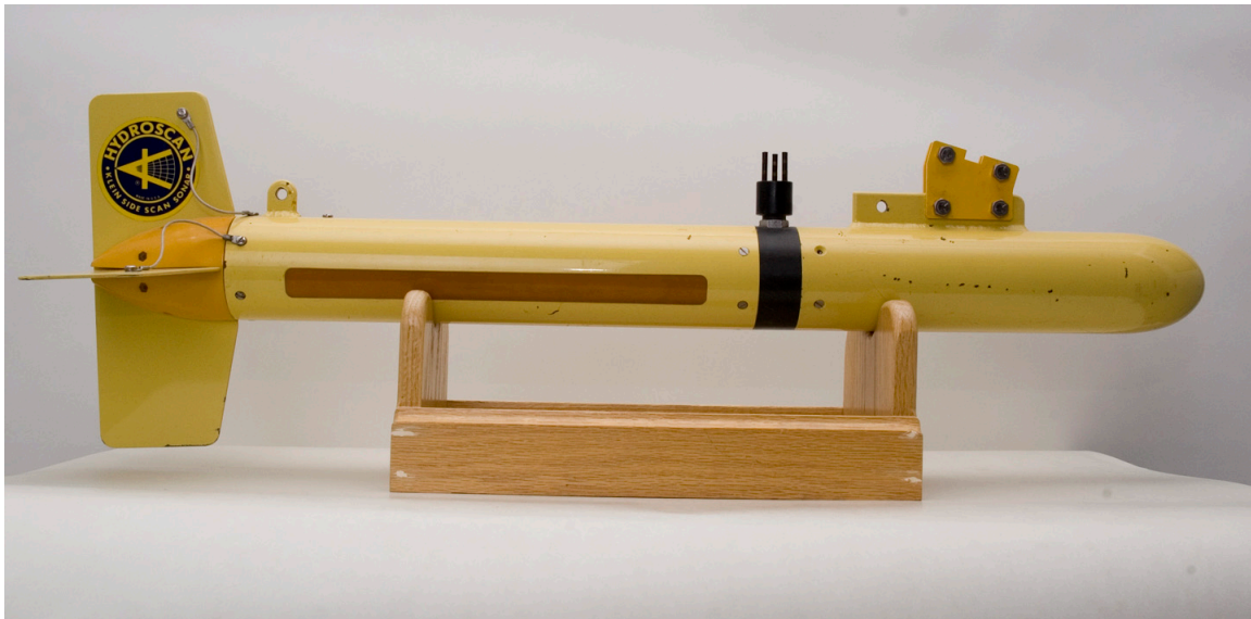
Prototype side-scan sonar designed by Martin Klein '62.
