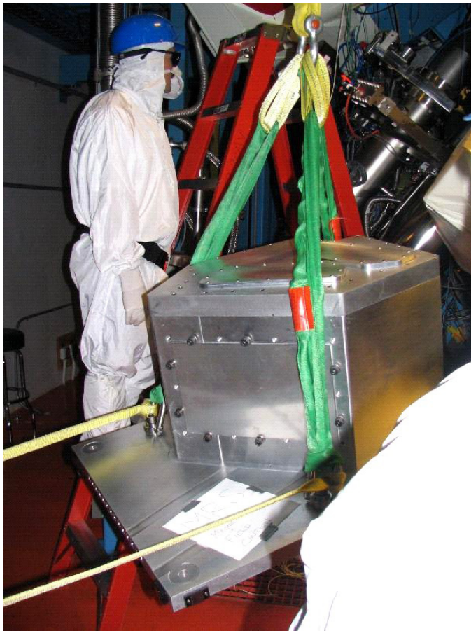
Figure 5. The spectrometer magnet enclosure just before being hoisted and interfaced to the OMEGA target chamber.
