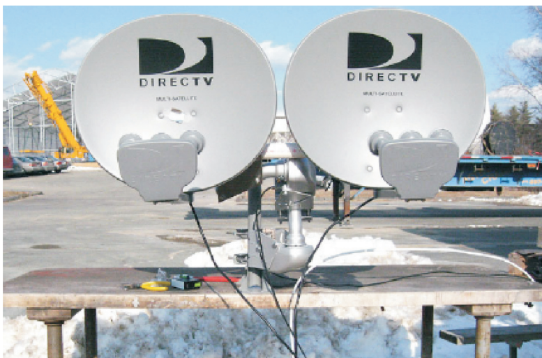
Figure 8. The very small radio telescope system at Haystack Observatory uses low-cost commercial satellite-TV dishes and receivers.
