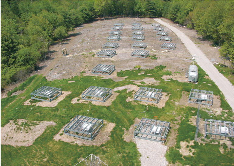
Figure 2. The deuterium array at Haystack Observatory as it existed from 2004 until July 2006. The trailer contains the radio frequency interference detection equipment.
