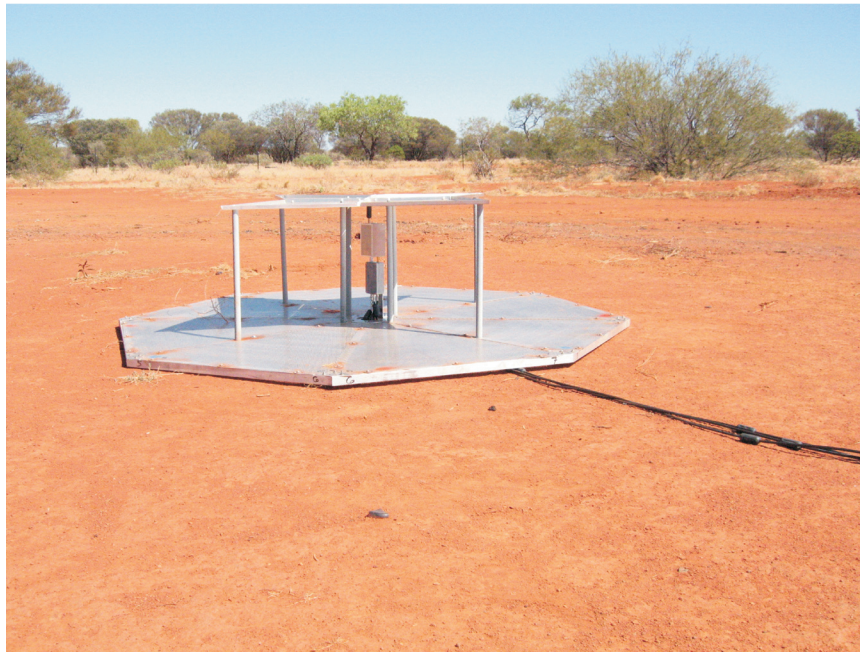
Figure 3. The EDGES antenna at Mileura Station in Western Australia in December 2006. The antenna and spectrometer cover a frequency range from 100 MHz to 200 MHz.
