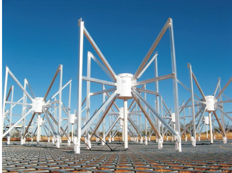
Figure 4. Manufactured antenna tile installed at Boolardy Station, Western Australia. The approximate cost per dipole is $50, and the associated rigid-wire mesh underneath it costs about $15 per dipole.
