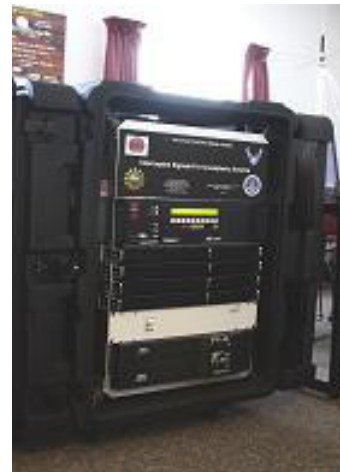
The ISIS mobile data acquisition system, developed for bistatic observations with incoherent scatter radar, passive radar, and distributed GPS receivers.
