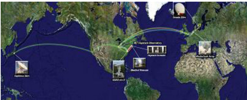
Demonstration of e-VLBI wideband data transport from international radio telescopes to the correlator at Haystack Observatory for real-time processing.
