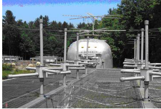
This close-up of one station of the deuterium array at Haystack shows the dual-polarized dipoles with beam directors. The trailer in the background contains the radio frequency interference detection system.
