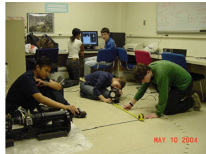
Students worked in the lab to calibrate ASIS with a light source to determine dark noise, relative spectra, and vignetting.
