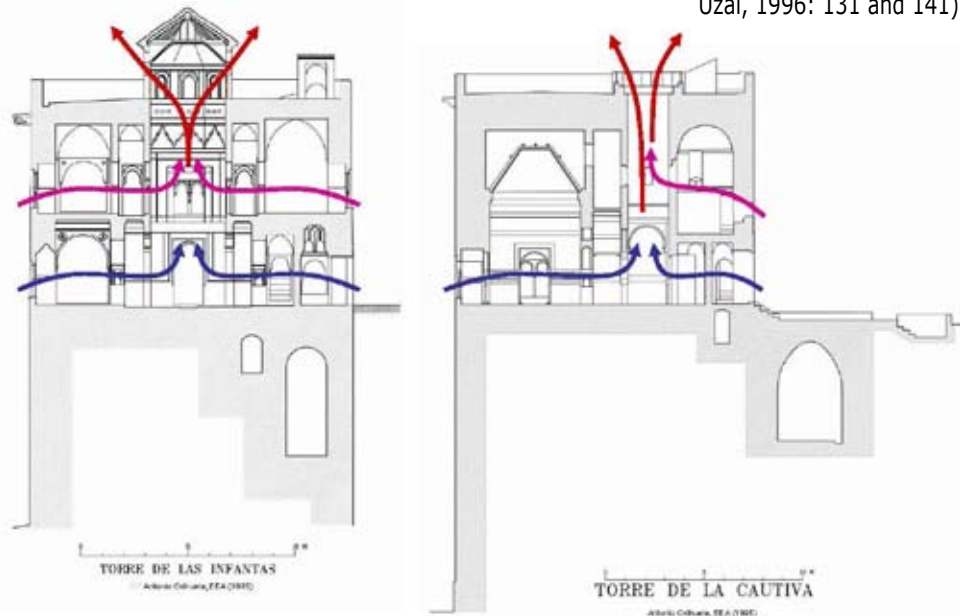
Image 6.5. Ventilation effect in the Las Infantas and La Cautiva towers-houses in the Alhambra (after maps from Orihuela Uzal, 1996: 131 and 141).
