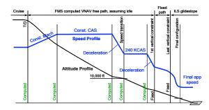
Figure 2: Vertical profile of RNAV CDA
