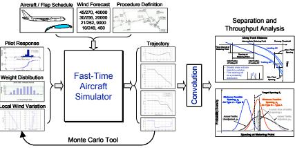
Figure 3: Tool for the Analysis of Separation And Throughput (TASAT)
