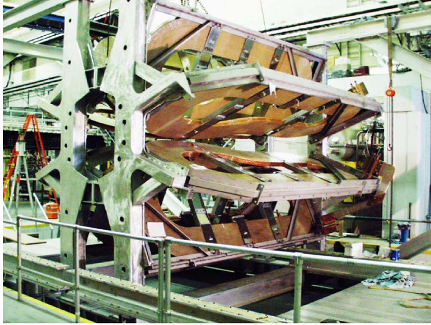
Figure 2.4: The eight coil BLAST toroid without its detectors.
