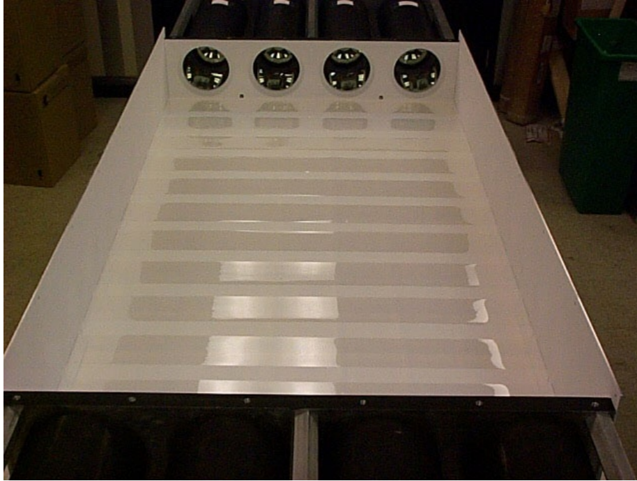
Figure 14: Inside view of Čerenkov detector showing white painted box with aerogel and openings for four PMTs.
