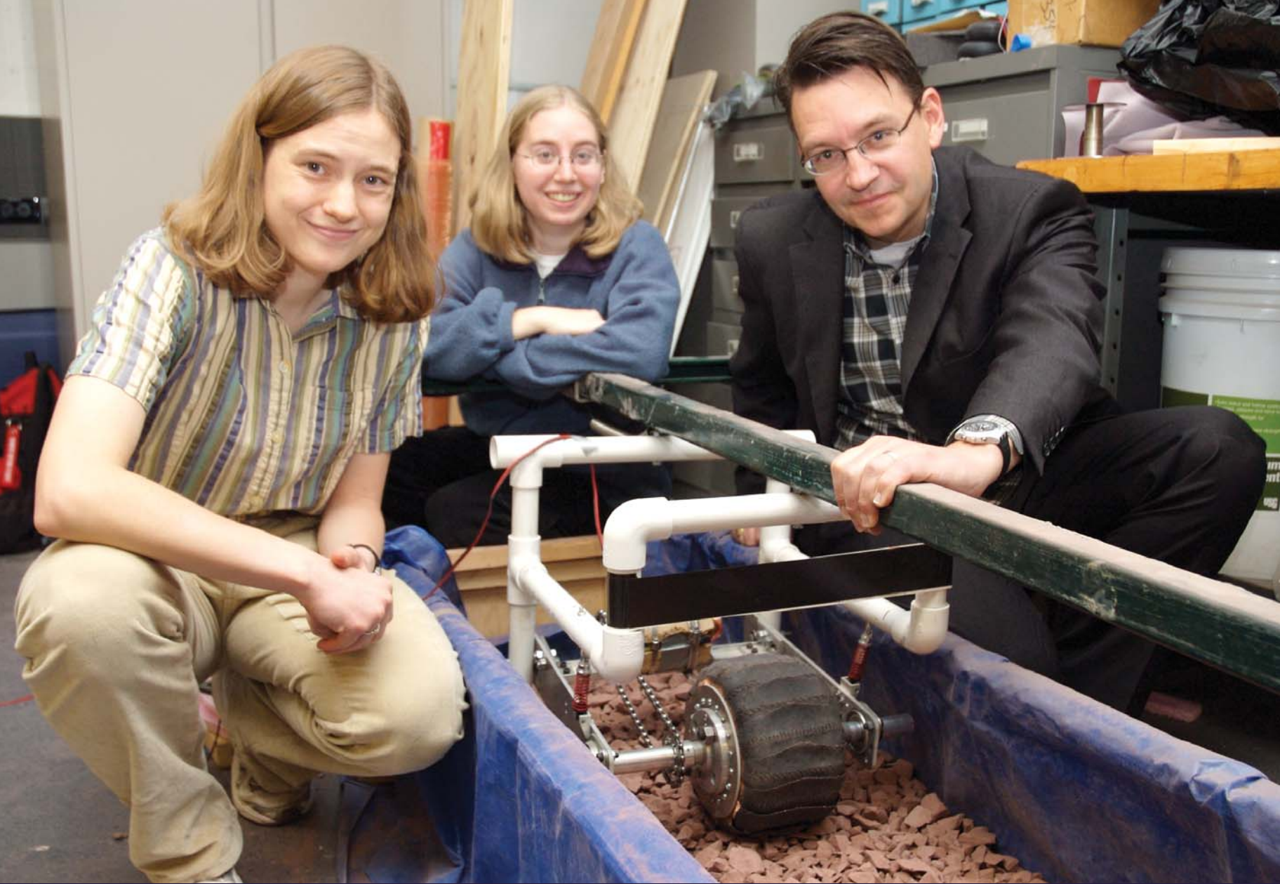
Olivier de Weck with Experimental Projects (16.622) course students Brittany Baker (left) and Noelle Steber in Aero-Astro's Gelb Laboratory with their planetary rover reconfigurable wheel testbed. The wheel can change its shape to optimize drawbar pull and power consumption for varying soil conditions. (William Litant/MIT photograph)
