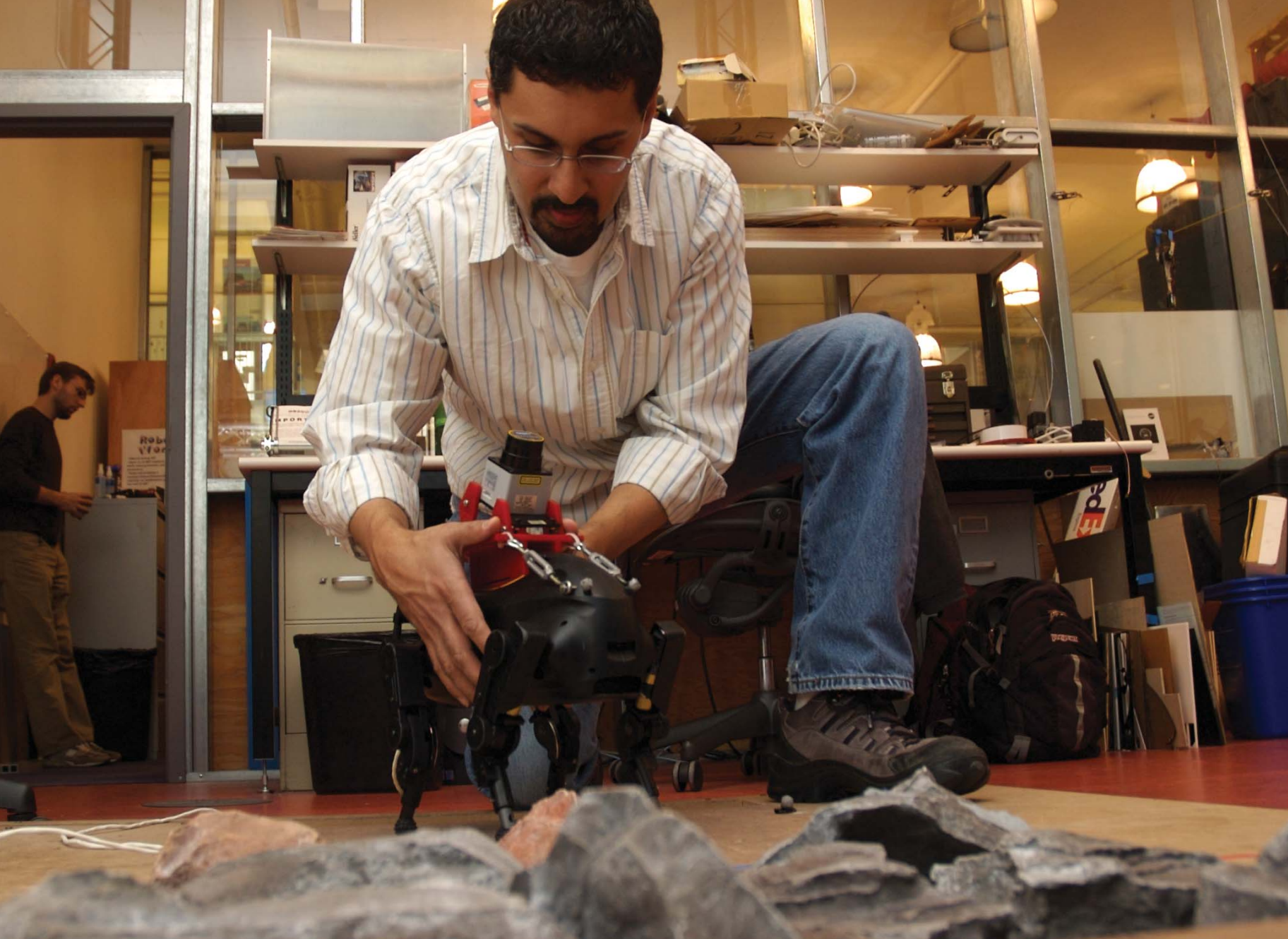
Nicholas Roy is developing intelligent estimation and planning algorithms that allow his robot dog to learn the shape of the ground via data from sensors such as the laser on its back. The dog applies the information to select footholds as it traverses rugged and uneven terrain. (William Litant/MIT photograph)
