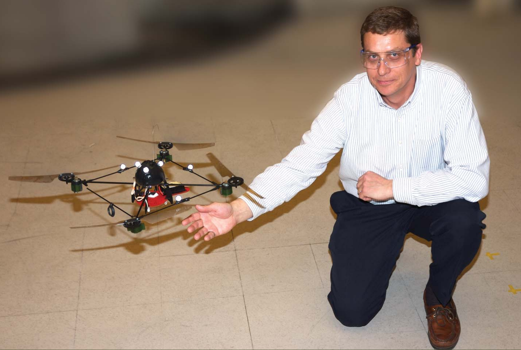
Its four rotors frozen by the camera, a quadrotor hovers above Aero-Astro Professor Jon How's hand. Flying autonomously, the UAV will stay within a 20 cm box-shaped space — a feat exceeding the capabilities of the best human pilots. (William Litant photograph)
