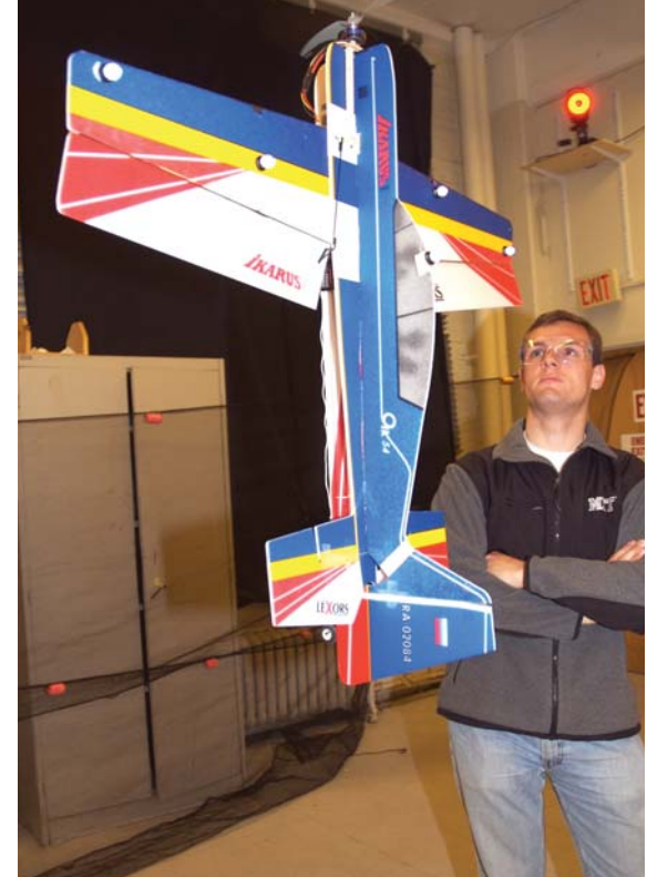
Graduate student Per Adrian Alexander Frank observes a foam aircraft as it autonomously hovers nose-up in the Aerospace Controls Lab — an extremely challenging, and successful, test. (William Litant photograph)
