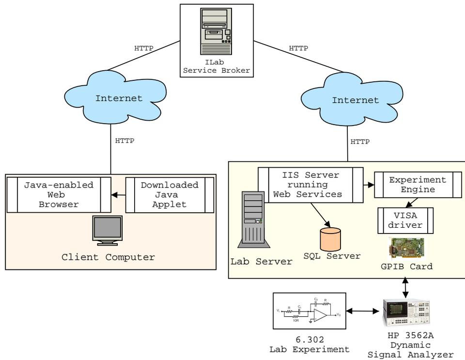
Figure 2-1: Architectural overview of the Feedback Systems WebLab Prototype
