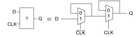
3) What is the setup time, hold time, and clock to Q delay of the above memory element?
