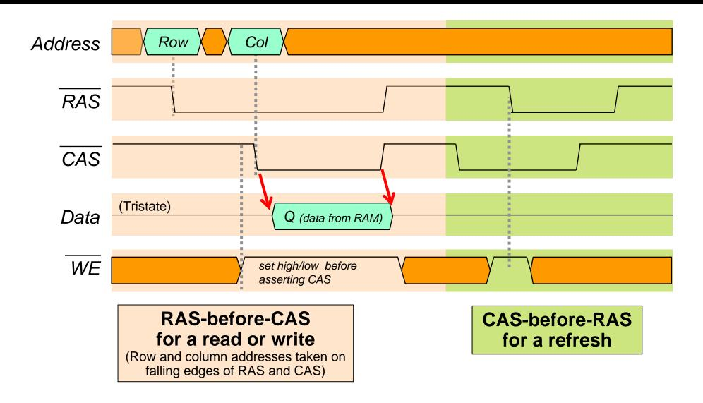
Clever manipulation of RAS and CAS after reads/writes provide more efficient modes: early-write, read-write, hidden-refresh, etc. (See datasheets for details)
