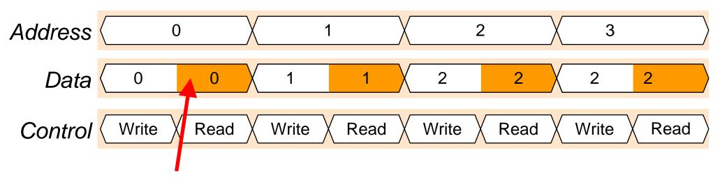
Data bus is undriven but wire capacitance briefly maintains the bus state: memory appears to be ok!
