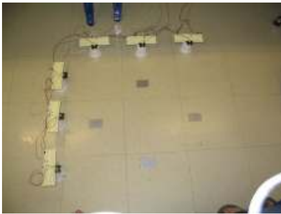
Figure 9: Picture of the grid created by the 6 infrared sensors.
