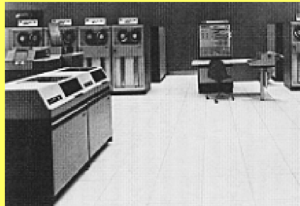
IBM System/360, 1964 500,000 adds/sec
