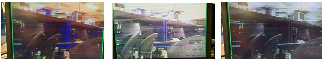
Figure 2 - Comparison of normal, high-brightness, and low saturation images from left to right (modified using I2C module for ADV7185 register control)
