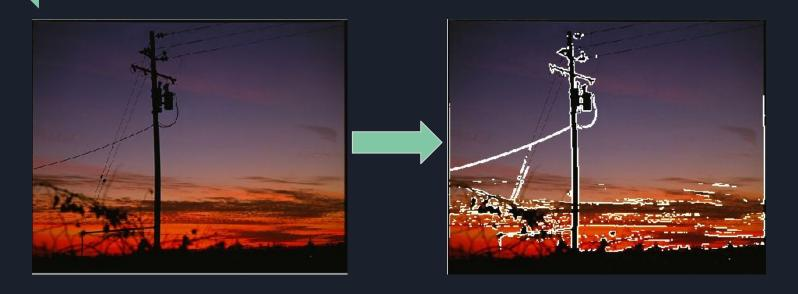
Sobel edge filter to highlight obstacle edges for better visibility
