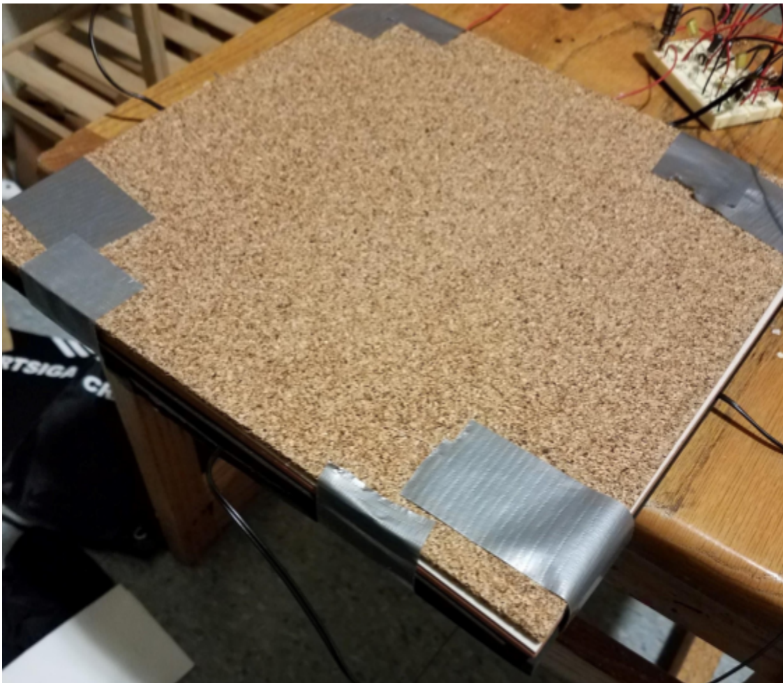
Photograph of the drum pad. The 4 piezo transducers were sandwiched between two ¼ inch layers of neoprene foam. A ceramic tile was placed on top of the foam to distribute the force of the drum hits, and a layer of cork board
