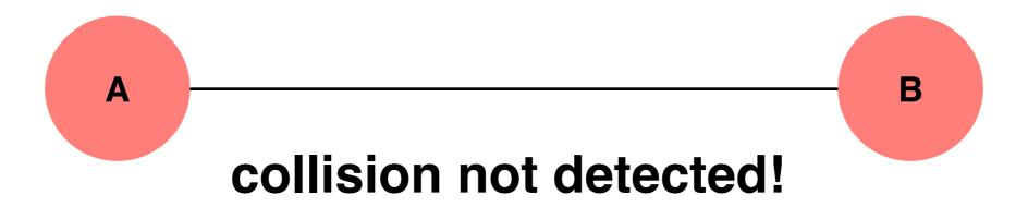
for collision-detection to work, endpoints must send for at least twice the latency of the link
