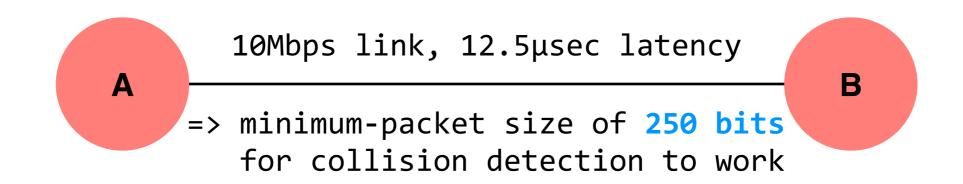
first ethernet standard: 10Mbps link, 12.5µsec latency, 112-bit packet headers
