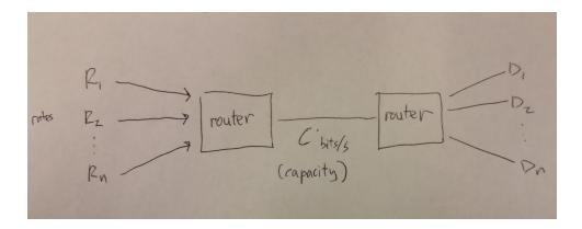
Suppose we have N sources, with source i transmitting packets at rates  $R_i$  bits/s via a router with a C bits/s link, as shown in the picture above. Then, congestion is said to occur when
