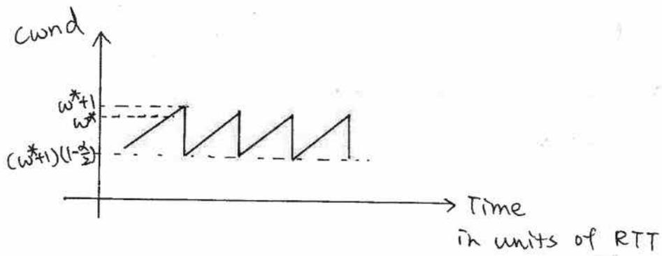
**Router** Marks all packet when  $Q \geq K$ .
