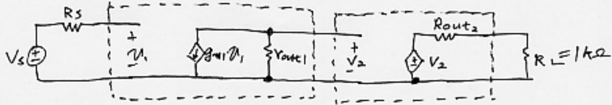
$$g_{m1} = \sqrt{2 \cdot M_n C_o \frac{W}{L} \cdot I_D} = \sqrt{2 \cdot 50 \mu \times \frac{40}{2} \times 50 \text{mA}} = 1 \text{mA/V}$$
