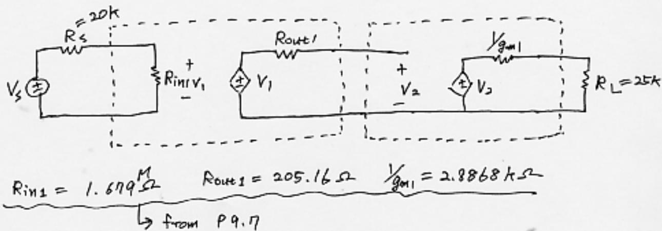
$$(d) \frac{V_{out}}{V_s} = \frac{1.679 \text{ M}\Omega}{1.679 \text{ M}\Omega + 20\text{k}\Omega} \cdot \frac{25\text{k}\Omega}{2.8868 \text{ k}\Omega + 25\text{k}\Omega} = 0.886$$
