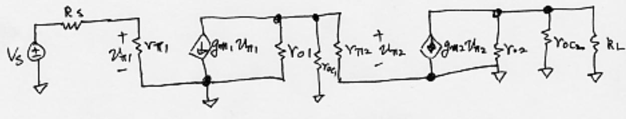
$$g_{m1} = \frac{100 \text{ mA}}{25 \text{ mV}} = 4 \text{ mA/V}$$
