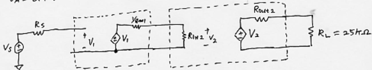
$$g_{m1} = \sqrt{2 \cdot \mu n C_o x \frac{W}{L} \cdot I_D} = 346.4 \text{ mA/V} \quad \therefore \frac{1}{g_{m1}} = 2.8868 k\Omega$$
