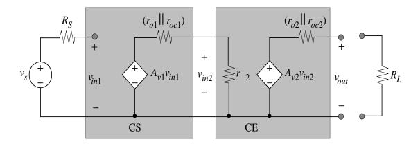
However, inter-stage loading degrades gain:
