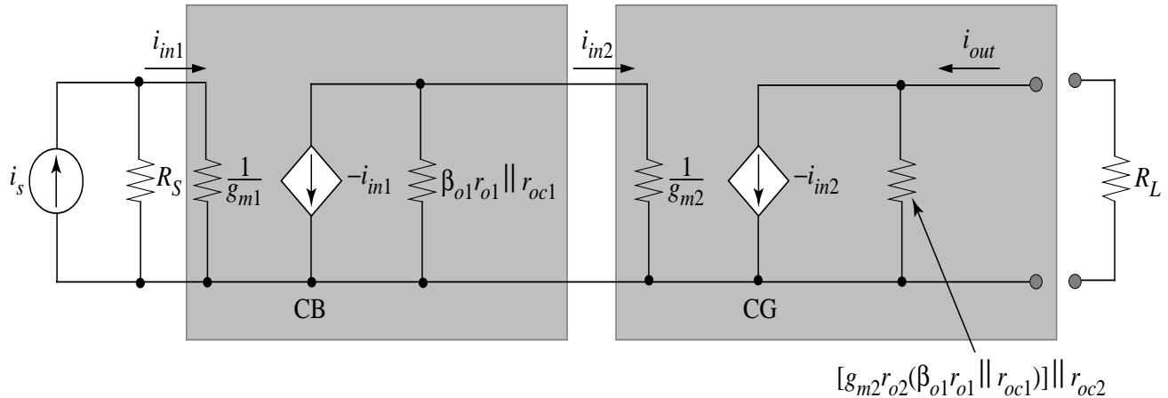
$$R_{out} = R_{out2} = r_{oc2} \parallel [r_{o2}(1 + g_m2 R_{out1})]$$
