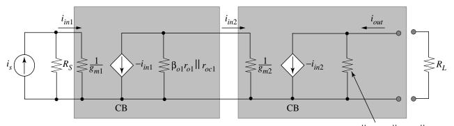
$[g_{m2}r_{o2}(r_{2} || \beta_{o1}r_{o1} || r_{oc1})] || r_{oc2}$
