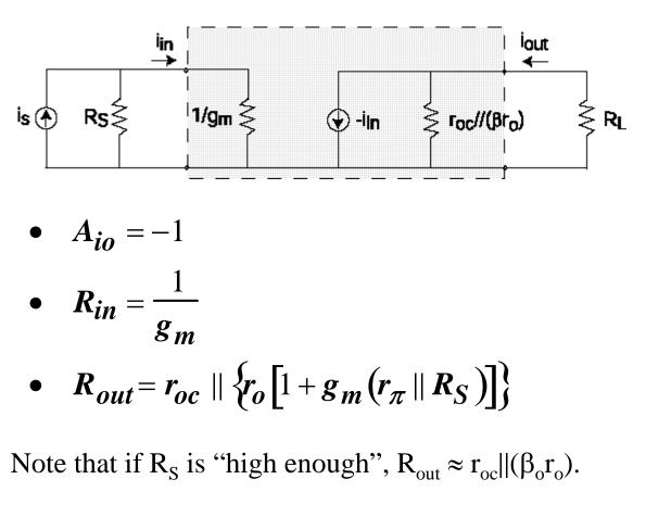
Can we increase R<sub>out</sub> further by adding a second CB stage?
