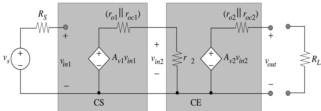
However, inter-stage loading degrades gain:
