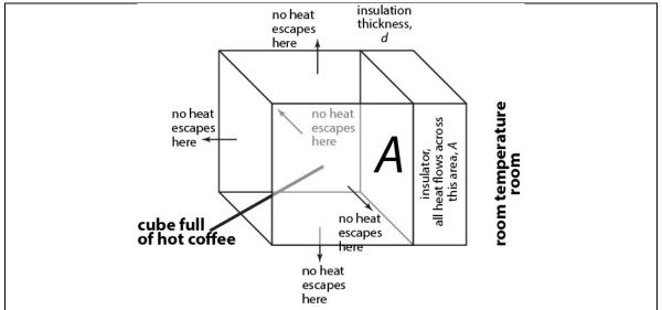
**Figure 2** A idealized coffee cup; heat is only lost through conduction in one direction across an insulator of cross-sectional area, *A*, and thickness *d*.
