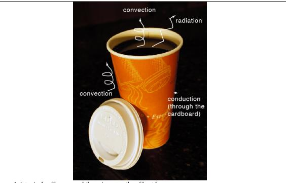
Figure 1 A typical coffee cup and the primary paths of heat loss
