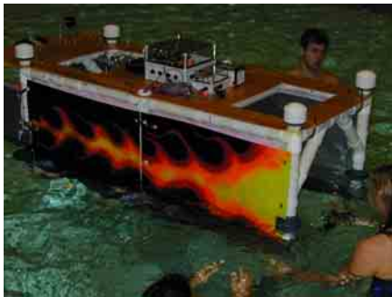
The SWATH being tested in the pool.
