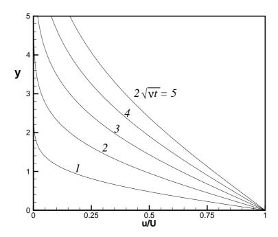
Figure 1.8.1: Velocity profile due to impulsive motion of x-plane
